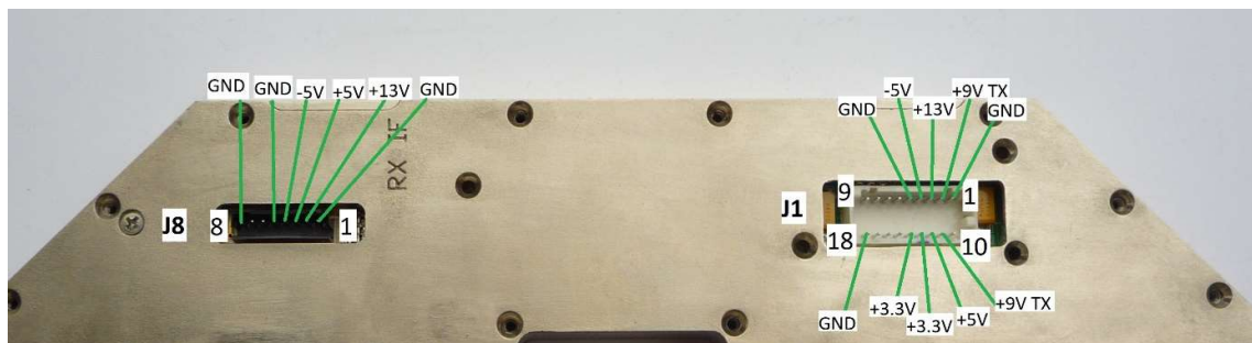
Figure 6. Power supply pins
